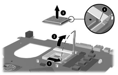
Removing the Processor
